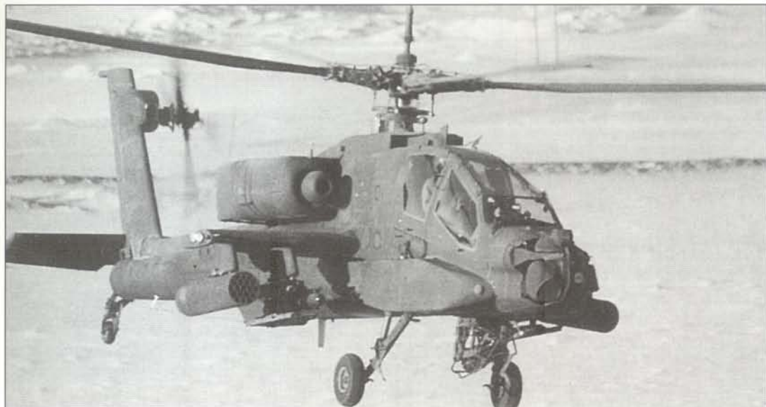
Carrying multi-tube rockets launchers and AGM-114 Hellfire anti-tank missiles in addition to the 30 mm Chain Gun cannon under the fuselage, the McDonnell Douglas AH-64A Apache proved itself wholly the master of Iraqi armoured formations
