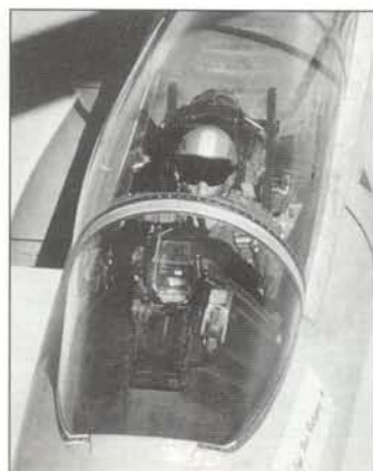
Seated on a zero/zero ejection seat with the screen of the HUD in his forward line of sight, the pilot of the McDonnell Douglas F-15C air-superiority fighter has excellent all-rounds fields of vision through the carefully designed canopy
