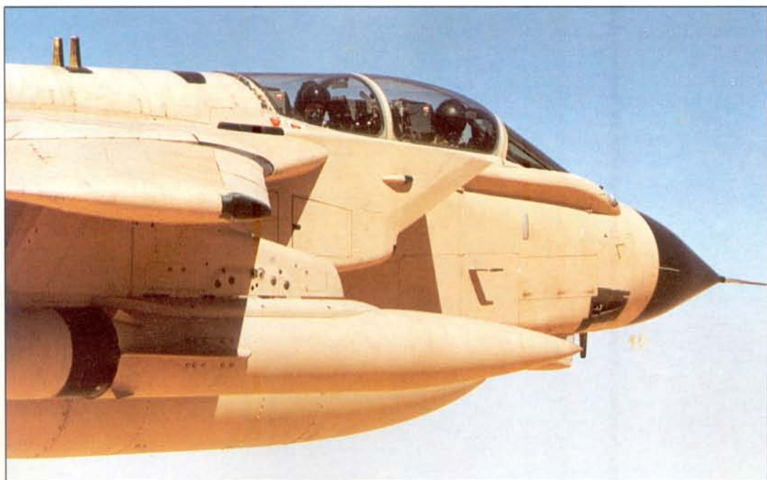
Visible on the forward fuselage of this Panavia Tornado GR.Mk 1 interdictor are the radome over the radar equipment, the dark surround of the muzzle port for the starboard 27 mm Mauser cannon, and the retracted inflight-refuelling probe.
