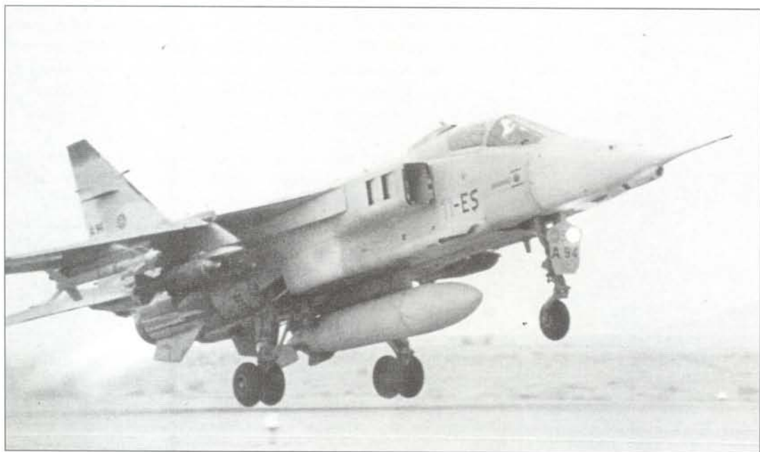
Fitted with a centreline drop tank and, under the wing, outboard AAMs and inboard 'iron' bombs, this Jaguar A of the French air force is taking off in full afterburner for an attack mission
