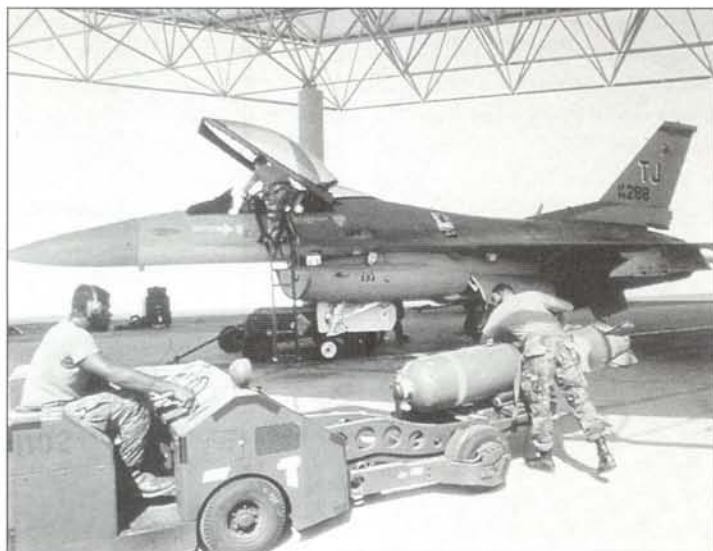
Protected from the harsh sunlight of the region but against little else, the General Dynamics F-16C Fighting Falcon was a workhorse of the American air effort. Here members of the ground crew bring up a Tactical Munitions Dispenser, a weapon that carries a mix of anti-armour and anti-personnel mines
