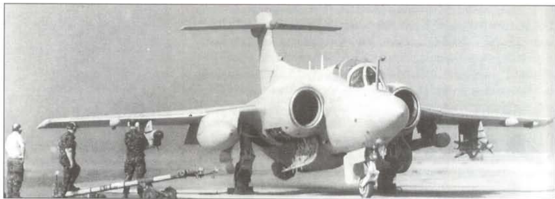
The BAe Buccaneer S.Mk 2B was in the last stages of its service life with the Royal Air Force when its capabilities were demanded in Saudi Arabia to provide laser illumination for the laser-guided bombs carried by other warplanes. Seen in the course of grounds tests at Muharraq, this Buccaneer carries four stores under its wing: from left to right these are ALQ-101(V)10 radar jammer, a slipper fuel tank, the AVQ-23E 'Pave Spike' laser pod (with its optics covered) and an AIM-9L Sidewinder short-range AAMs for self-protection
