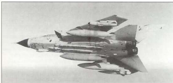
The Tornado F.Mk 3 air-superiority fighter's counterparts were the Tornado GR.Mk 1 long-range interdicator and, as seen here, the Tornado GR.Mk 1A reconnaissance type. Provided by either No. 2 Squadron at Laarbruch in Germany, this has a horizon-to-horizon IR system in place of the interdicator's two 27 mm cannon, and in addition to two drop tanks carries under the port and starboard halves of the wing a Marconi Sky Shadow ECM pod and a BOZ-107 chaff/flare dispenser pod respectively
