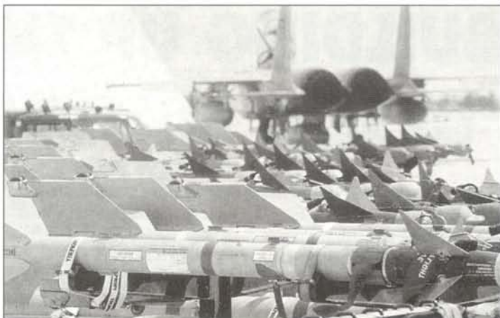
The standard short-range weapon carried by the McDonnell Douglas F-15 Eagle and other American fighters was the AIM-9M Sidewinder missile, an effective missile with all-aspect engagement capability
