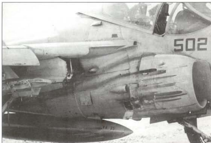
The coalition air forces did not have things all their own way, as suggested by the damage to this Grumman A-6E Intruder. Hit by ground fire, the aeroplane returned to its parent carrier with its two crew members unharmed, but was later scrapped
