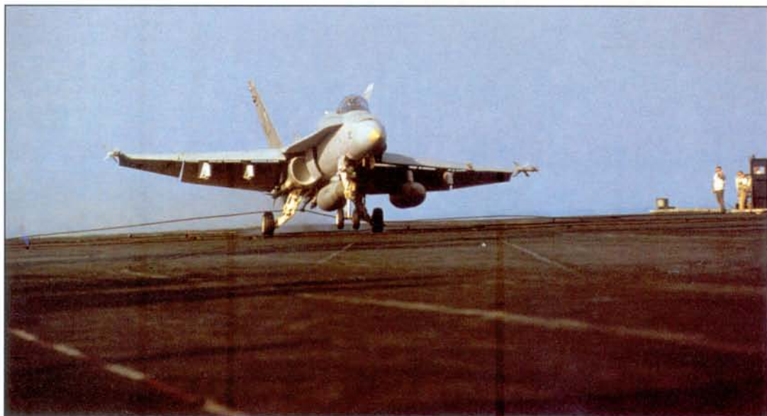
Flaps, landing gear and arrestor hook lowered, a McDonnell Douglas F/A-18 Hornet prepares to touch down on its flight deck of its parent carrier. The Hornet was notably important for air operations over Iraq, for it was a dual-role type that could operate as a fighter and an attack warplane as the situation demanded.
