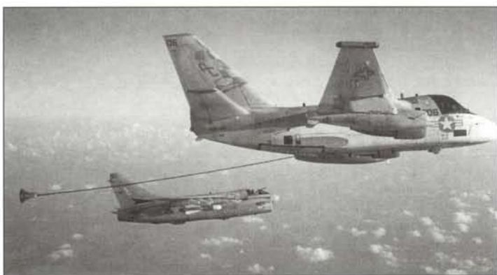
With no submarine threat to guard against, the Lockheed S-3 Viking could be adapted for other tasks. Here an S-3B of the USS John F Kennedy 's VS-22 squadron is operating in the 'buddy' tanker role with a hose-and-drogue unit to refuel one of a Vought A-7E Corsair II squadron
