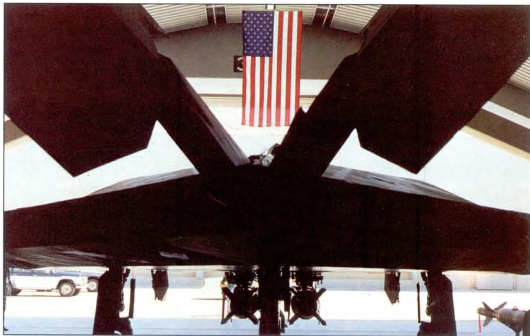
Seen here with two bombs extended below the pair of side-by-side weapons bays in the lower fuselage, this is the first Lockheed F-117A Night Hawk to arrive at Khamis Mushait Air Base in Saudi Arabia.
