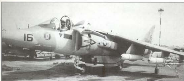
Close air support for the ground forces of the US Marine Corps was provided by the McDonnell Douglas/BaE AV-8B Harrier II, a STOVL warplane able to operate from shores offshore or beach-head airstrips immediately behind the front line
