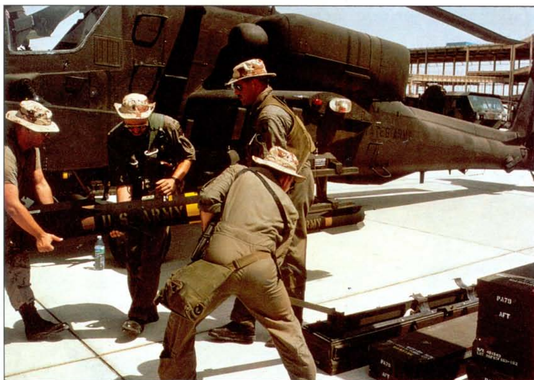
Men of the US Army's 101st Airborne Division load AGM-114A Hellfire anti-tank missiles on a hardpoint under the stub wing of one of the divisional air brigade's McDonnell Douglas AH-64A Apache anti-tank helicopters.
